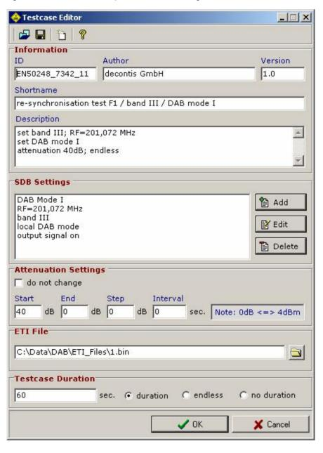
Fig. 3-1: DAB Test Client - Testcase Editor
