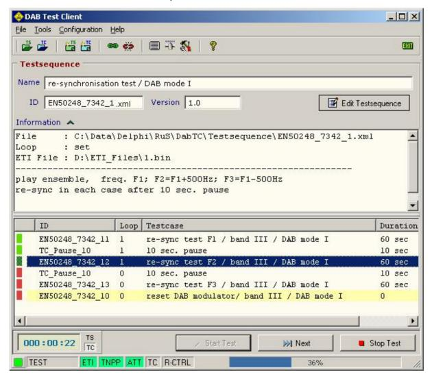
Fig. 4-1: DAB Test Client processes the test-sequence
